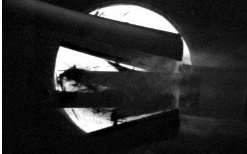
Fig. 9 Visible light image of fractured carbon-carbon projectile in flight
