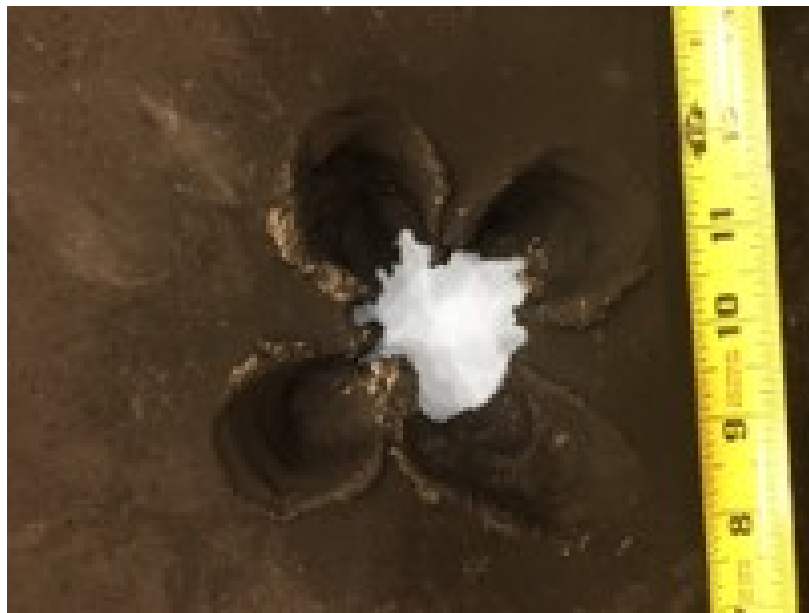
Fig. 11 Impact of Sabot hitting striker plate too close to pass-through
